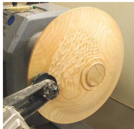
▲ Pic.12 Carve the bowl with the lathe stationary. Try and keep both hands on the tool until you become proficient at working the tool safely. Dabbing the tool against the surface works best
